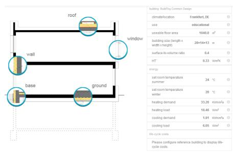
Changes to the building envelope system can have undesired and sometimes detrimental effects to the moisture-temperature gradients in the envelope systems. The BEG does provide limited information (see below as an example). It is advisable to engage a knowledgeable building physics expert/ buildings services engineer to evaluate proposed changes.
